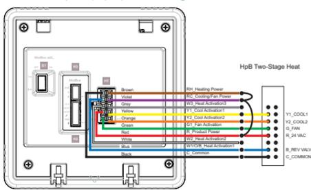
Heat Pump O (HpO) Two-Stage Heat: 24 VAC
