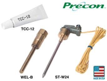
The thermowells are designed with close tolerances, eliminating the need for thermal grease under normal conditions. Each well is designed so that the sensor assembly can be easily removed after installation. The well screws into a 1/2" FNPT saddle (or Thredolet® fitting) furnished by the installing contractor.
