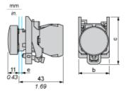
e: clamping thickness: 1 to 6 mm / 0.04 to 0.24 in. b: 30 mm / 1.18 in.
