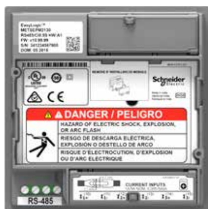
Rear of PM2000 without I/O module
