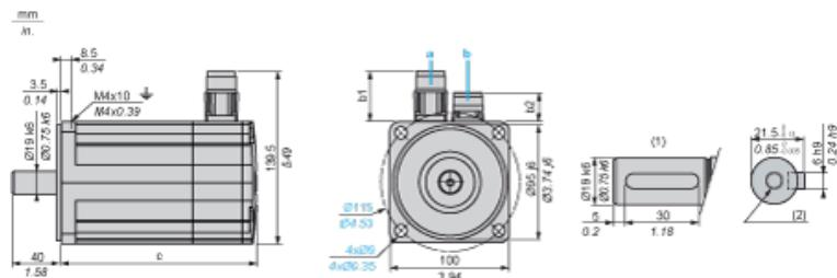
a: Power supply for servo motor brake
