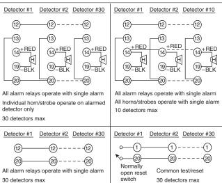
**NOTE:** When using detector interconnection functions, wire all detectors to a common power source. Use of multiple power sources for interconnected detectors may cause damage to the detectors and/or may prevent the detectors from functioning properly.
