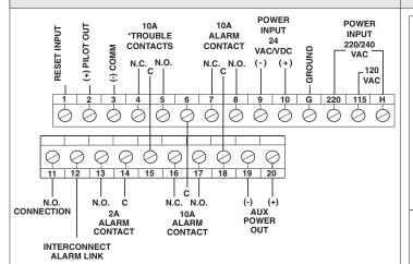
\*Trouble contacts are shown in non-energized condition. Under normal operation contacts will be reversed.
