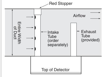
Note: Sampling tubes over 3' (0.9m) must be supported on the opposite side of the duct from the detector.
