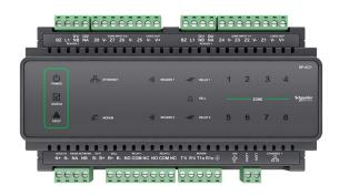
The Security Expert LON Controller is the central processing unit of the Security Expert System. It communicates with all system modules, stores all configuration and transaction information, processes all system communication, and reports alarms and system activity to a monitoring station or remote computer.
