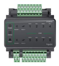
The Security Expert 2 Door Mini Expander provides the interface of up to 4 reader inputs and 2 locking device outputs to the Security Expert system, an advanced technology security product providing seamless and powerful integration of access, security and building automation. The Door Expansion provides extensive hardware advancements that provide flexible access control, area control and alarm monitoring, and is designed for use with industry standard DIN Rail mounting or wall mounting.
