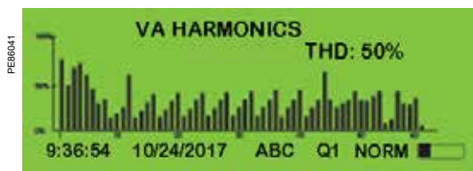
PowerLogic ION8650 front panel harmonic display.
