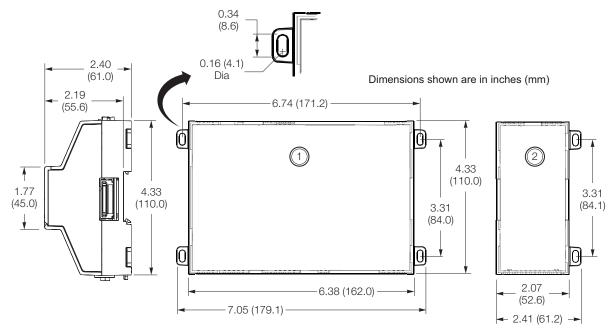
Compatible with (DIN43880) enclosures. Suitable for mounting to a panel or to an EN50022 standard 35mm rail.
