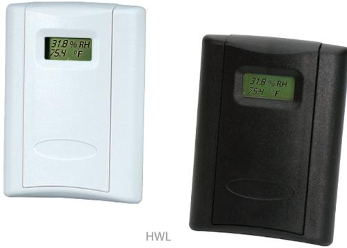
HW Series deluxe humidity transmitters provide an ideal solution for measuring relative humidity in all conditions. All devices are equipped with a thin-film capacitive sensor that is easily replaceable in the field. These sensors are calibrated to NIST standards, with certificates available (see Ordering Information; choose "N" in NIST block). Temperature sensing options are also available.
