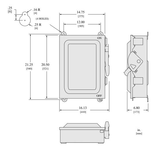
WHEN MOUNTING THESE SWITCHES, ALLOW 3.75/[95] MIN CLEARANCE BETWEEN ENCLOSURES FOR OPENING OF SIDE HINGED DOOR.
