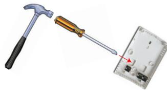
4. Position the backplate vertically on the wall, 4 ½ feet (1.4 m) above the floor. Locate away from windows, vents, and other sources of draft. If possible, do not mount on an external wall, as this might cause inaccurate temperature readings.
