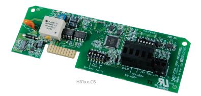
With the optional H81xx Communications Board, the H81xx Series energy meters connect easily to control/data systems networks using Modbus, BACnet, and Metasys (N2) protocols. The H81xx-CB reports energy and power diagnostic information including kW, kWh, kVAR, PF, amps, volts, and more.
