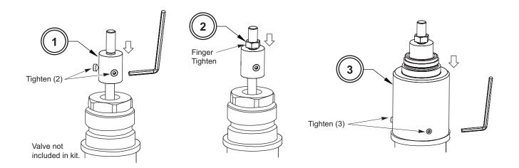
After the AV-814 adapter is installed, install the selected actuator and linkage (if required) according to the actuator installation instructions.
