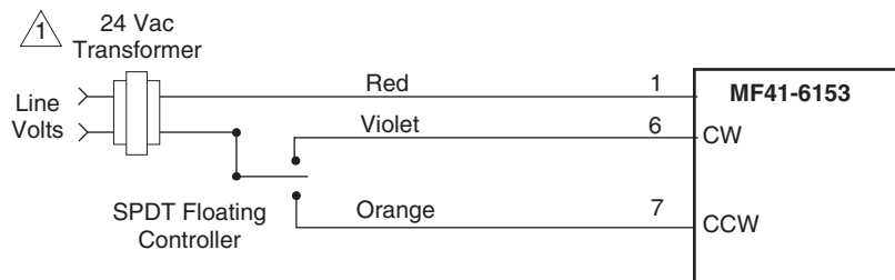
Figure 1 Typical Wiring Diagram for MF41-6153 Floating Actuators.
