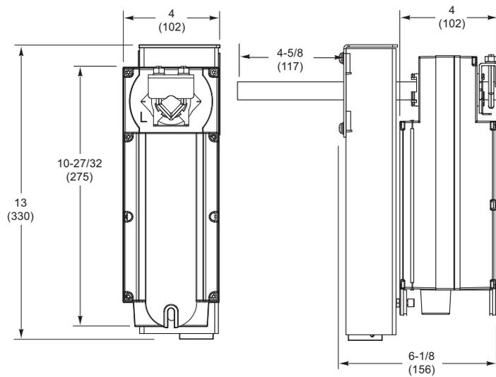
Figure-21 Mx41-6343 Actuator/Linkage Assembly With AV-609-1 Linkage.
