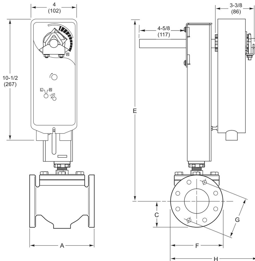
Figure-32 Mx41-715x or Mx41-707x with 2-1/2" to 4" 2-Way Flanged Globe Valve with AV-607-1 Linkage. Mx40-715X with 5" and 6" 2-Way flanged Globe Valve with AV-609-1 linkage
