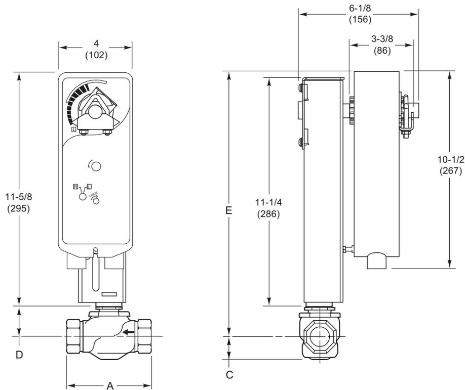
Figure-26 Mx41-715x or Mx41-707x with 1" to 2" 2-Way Globe Valve With AV-602 Linkage.
