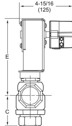
Figure-8 Mx41-6043 or Mx41-6083 with 2-Way Globe Valve with AV-611 Linkage.
