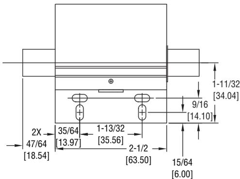
Figure 2: Mounting Hole Dimensions
