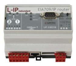
An L-IP redundant EIA-709/IP router can be used as a single device to achieve redundancy on the ANSI/EIA-709 (TP/FT-10) channel by building a ring structure. If IT network redundancy is available, full redundancy on the IP-channel and on the ANSI/EIA-709 channel can be achieved with two devices installed in parallel. In this case device redundancy is ensured as well by mutual monitoring of paired L-IP redundant routers.
