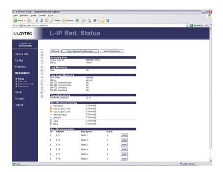
Without using an LNS plug-in the L-IP redundant EIA-709/IP router can be configured via the built-in web server, which also shows the health status of the TP/FT-10 ring and the connected nodes.
