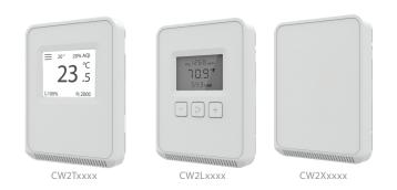
The CW2 Series of air quality sensors for living space is a flexible multi-sensor platform for use with BAS controllers designed to accept 4 to 20mA, 0 to 5Vdc or 0 to 10Vdc outputs. CW2 Series sensors are available with three user interface options: touchscreen, LCD with three buttons and blank.  $\rm CO_2$  and temperature sensors are included with all CW2 Series air quality sensors. Models with VOC sensors and relative humidity sensors are also available.
