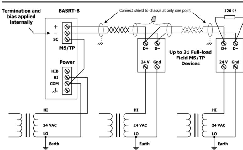
Figure 10 — 3-wire MS/TP Bus with Separate Power Sources
