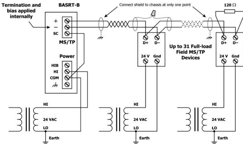
Figure 9 — 2-wire MS/TP Bus with Separate Power Sources
