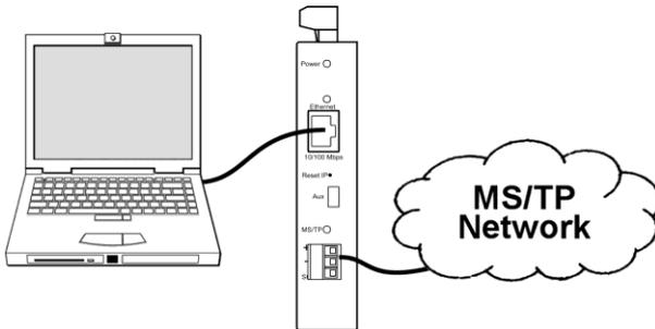
*Figure 12 — Setup for Initial IP Address Configuration*
