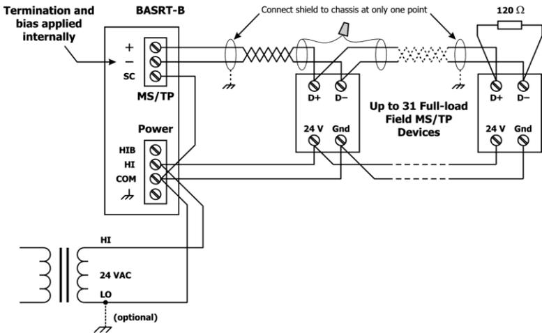
Figure 7 — 2-wire MS/TP Bus with Shared Power Source
