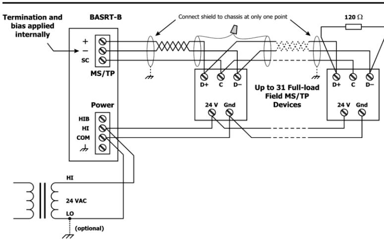
Figure 8 — 3-wire MS/TP Bus with Shared Power Source
