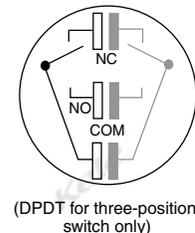
Non-Illuminated Push Buttons and Selector Switches (DPDT for three-position switch only)
