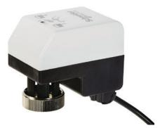
Reliable longtime operation is ensured from no mechanical feedback potentiometer and no mechanical end switches. Automatic synchronization function provides self adjusting close off. Based on a full stroke running time of 100 s, valve positioning and flow adjustment is very exact.
