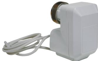
The MZ09L small linear actuator is specifically designed to provide LonMARK® capabilities together with radiator valves and is used in fan coil units, induction units, small reheaters and recoolers, and for zone control applications. The MZ09L actuator is suitable for LonWORKS technology. Using standard Echelon configuration tools, the actuator can be configured with job specific settings.
