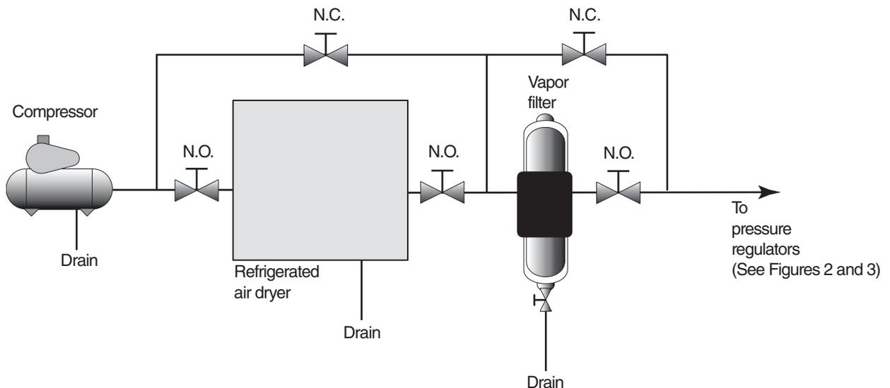
Figure-1 Recommended Air Supply System.
