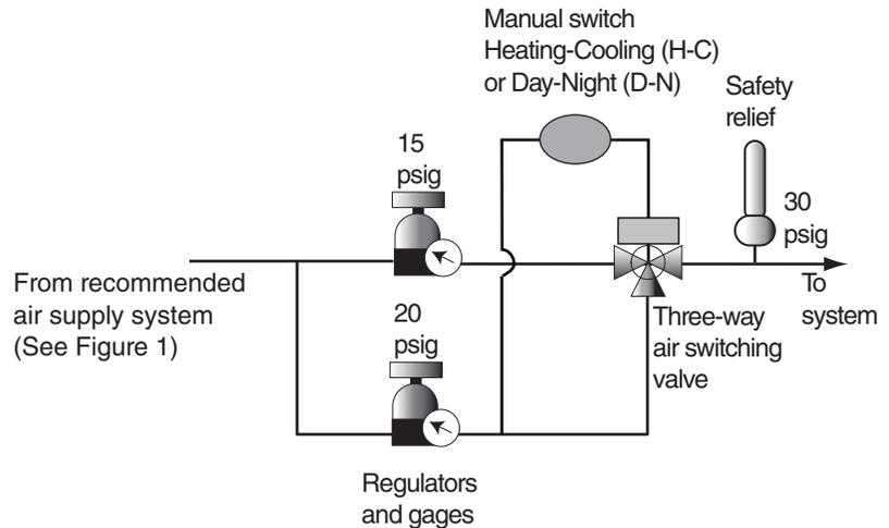
Figure-3 Dual Pressure System.
