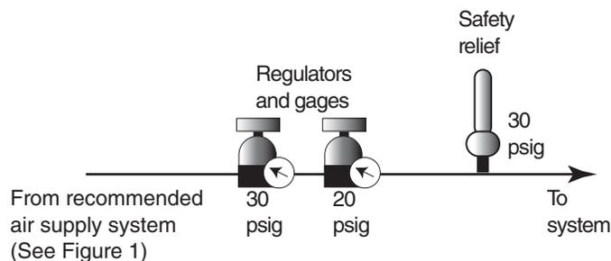
Figure-2 Single Pressure System.
